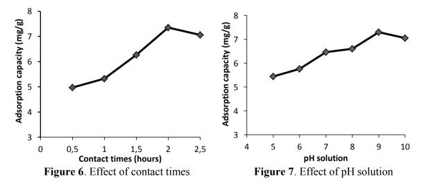
The effect of contact time on the adsorption of procion red dye by alumina-activated carbon composite was shown in figure 6. The adsorption process is influenced by the contact time. The contact time from 0.5 until 2 hours (interval 0.5 h) was increased the adsorption capacity and reached to equilibrium in 2 hours. The longer of the contact time, the more collisions between the dye and composite so adsorption capacity increases to reach equilibrium.
