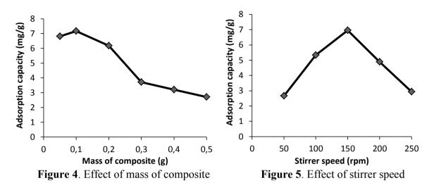
The effect of stirrer speed on the adsorption procion red dye onto composite that is presented in figure 3. At low stirrer speed, the effect of mass transfer for dye is increased the adsorption capacity. As the stirrer speed increases from 50 to 150 rpm, but at higher speed the adsorption capacity had lower. At high speeds, the number of collisions caused the release back the dye. In this study, the subsequent experiment are conducted at 150 rpm.
